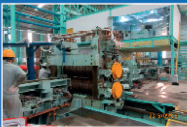
650 Two-high Reversing Mill Used for rolling of special alloys such as titanium alloy and nickel alloy
