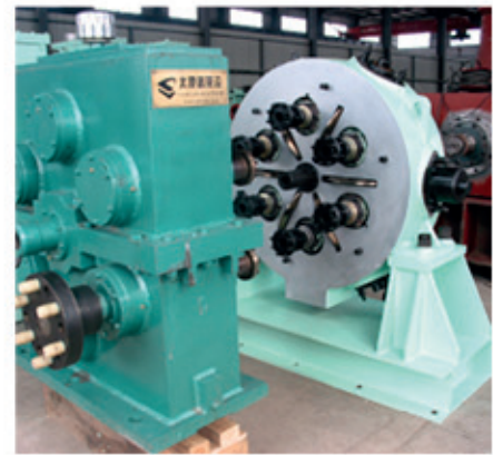
Six-Roll Mill Used for rolling hexagonal quadrangular brazed steel B19-B36
