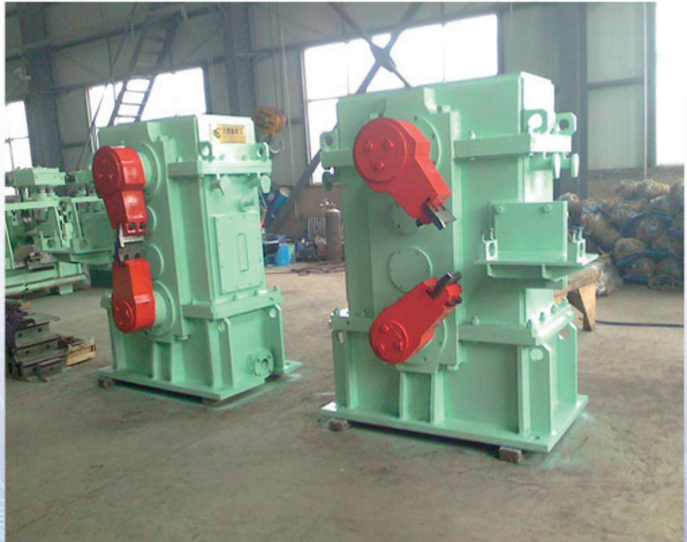
No 2 Flying Shear Used for cutting head and tail of wire rod and chopping
